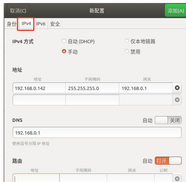
Figure 1-21 Configuring static IP address information
