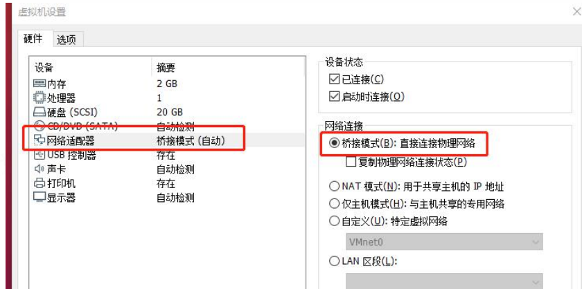
Figure 1-13. Changing the network connection mode of the virtual machine
